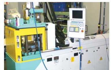
Injection molding for watertight sealing of submersible integral cables, cable strain relieving boots & sensor accessories
