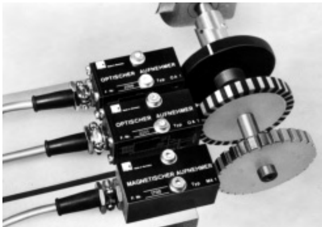
Fig. 8.4-15: Transducer systems for the non-contact acquisition of the speed of rotating parts
