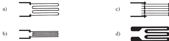
Fig. 3.3-5: Various shapes of strain gage measurement grid and methods of reducing the transverse sensitivity.
