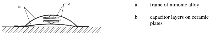
Fig. 1.0-11: Diagram of a capacitive strain gage from CERL-Planer.
