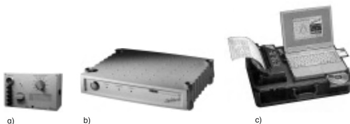
Fig. 6.4-1: Arrangement of the calibration unit within the measurement equipment. a) calibration unit b) measuring amplifier c) indicating instrument
