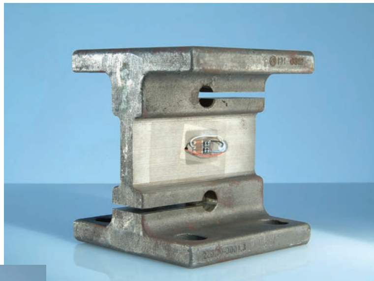
SG installation on customized machine element
